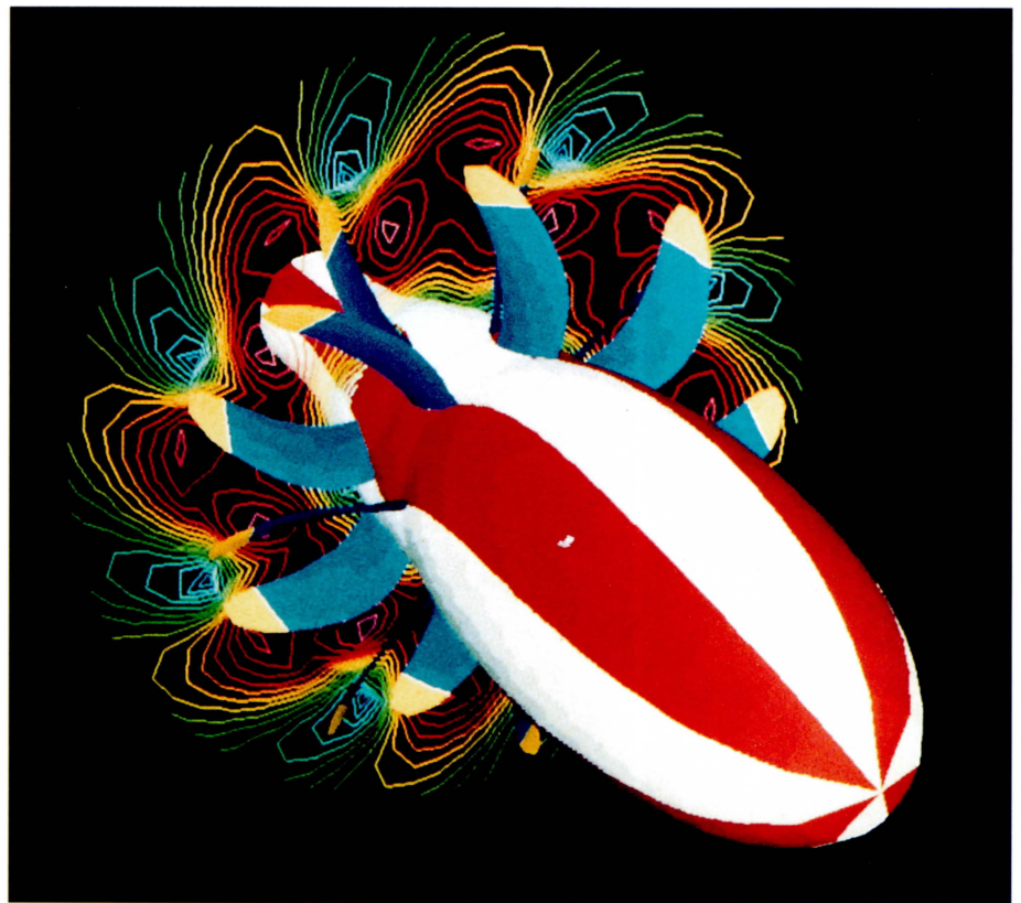
NASA's Lewis Research Center is using computational fluid dynamics to obtain a full three-dimensional solution for the unsteady flow field of counterrotation propellers. This figure of a General Electric Unducted Fan shows pressure contours in a plane just downstream of both blade rows. The blue areas represent lowest pressure contours and the pink represent the highest.
